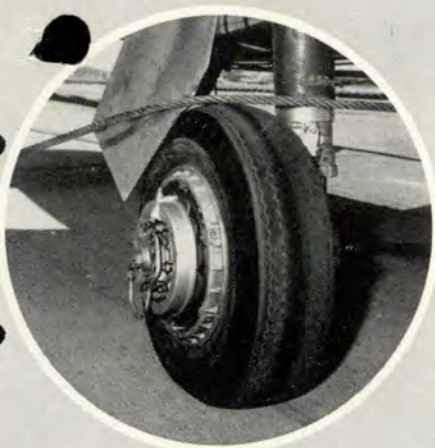
Here are some shots of the F-100 and landing gear struts. The tests were run at various speeds and in various configurations to determine the adaptability of the aircraft to the standard MA-1A barrier. The aircraft proved itself okay.
