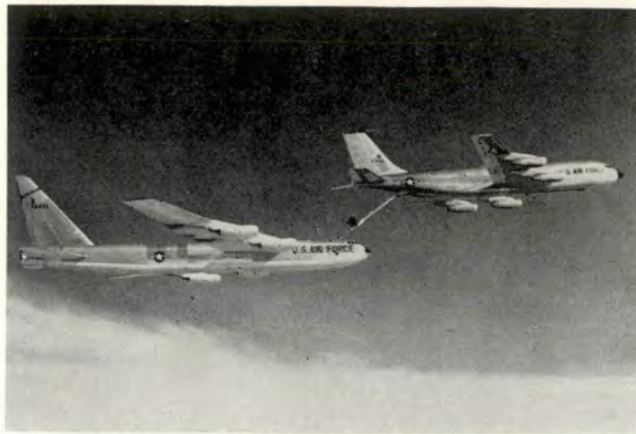
Above, shows the first KC-135 during initial aerial refueling tests.
